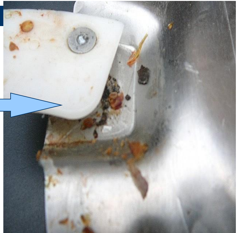
Non-removable, non-cleanable white plastic on inside of blade guard was Salmonella + PFGE match to outbreak
